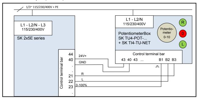
DIP switch settings (SK 2x5E - S1): DIP3 = off, DIP4 = on, DIP5 = off
