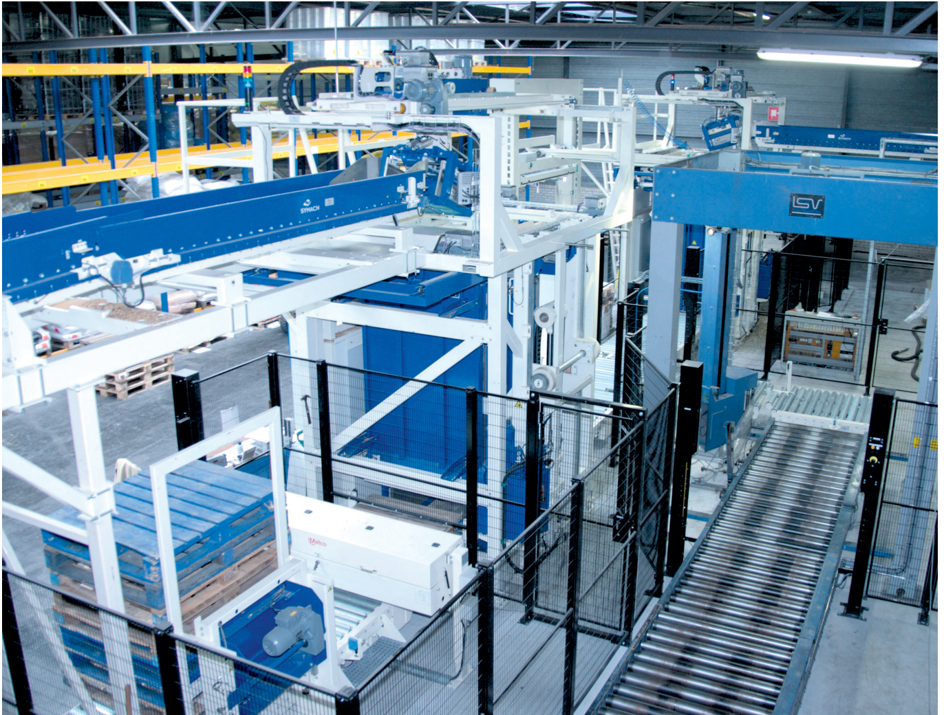
Palletizing machine with decentrally controlled asynchronous drive systems
