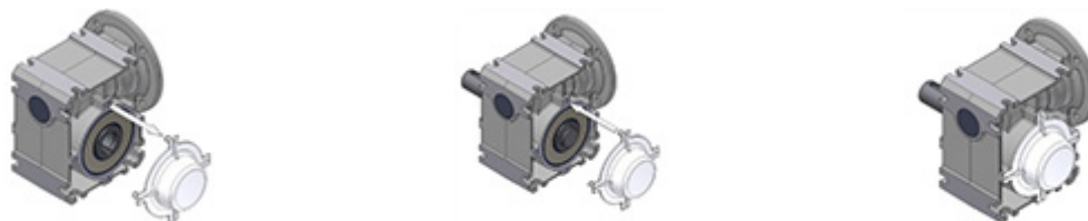
Figure 15: Disassembly and assembly of the cover cap
