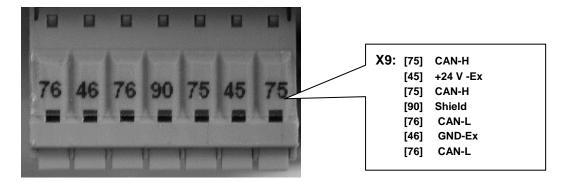
Terminals 75 and 76 on the spring terminal bar X9 are for connection of the signal leads from CAN High and CAN Low and are doubled for looping.
