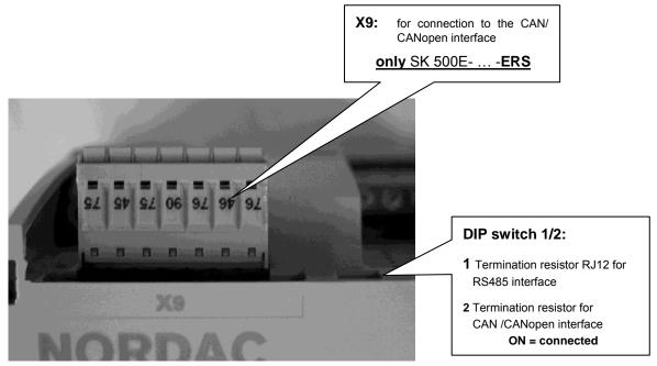
The 7-pin Phoenix spring terminal bar X9 (CAN plug) is used instead of the two RJ45 plug connectors (from SK 520E).
