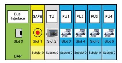
Figure 15: Example – PROFINET IP / PROFIsafe device model for decentralised devices
