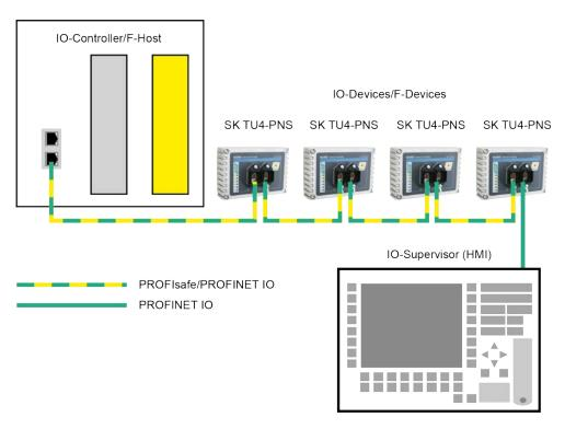
Figure 3: Linear topology (example)
