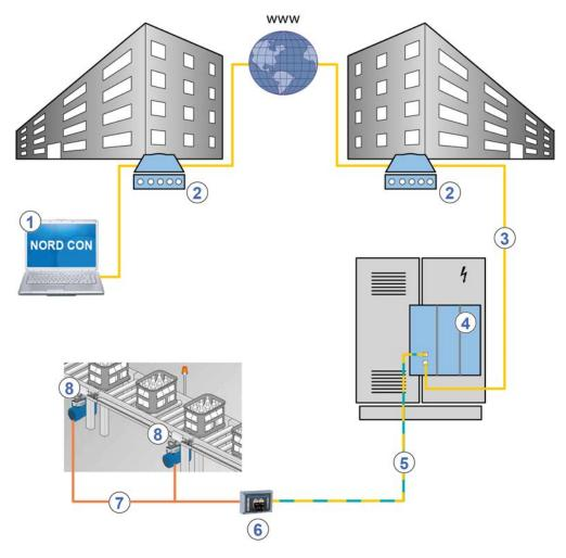
Figure 13: Remote maintenance via Internet (schematic diagram)
