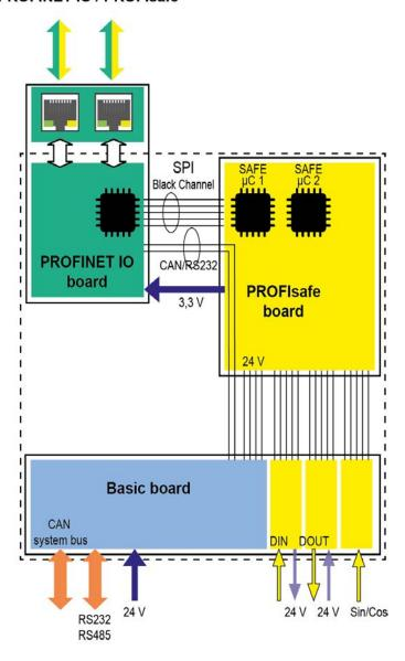
Figure 10: Bus interface - hardware
