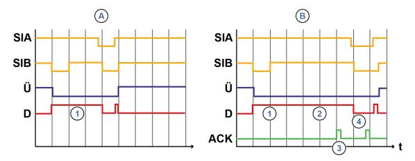
Figure 11: Monitoring of discrepancy time
