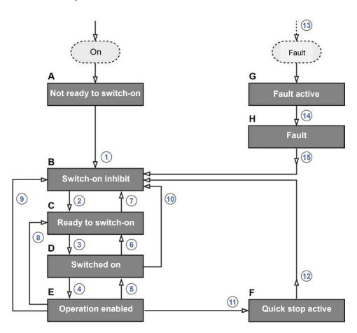
Figure 16: Frequency inverter status machine
