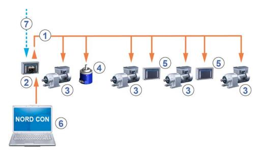
Figure 12: Example of the structure of a NORD system bus
