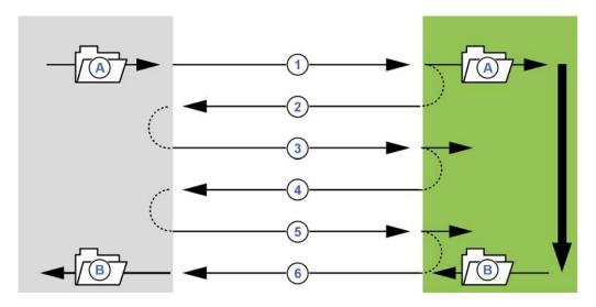
Figure 17: Sequence of acyclic PROFINET IO parameter data exchange
