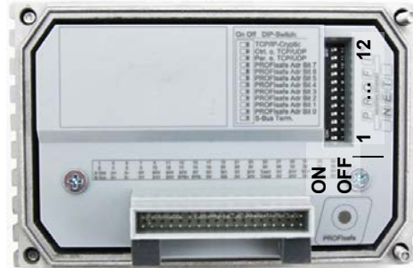
Factory settings DIP switches: OFF
