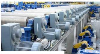
Parallel shaft geared motors for rolling mills
