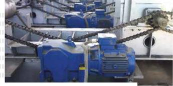
Bevel geared motors for cooling bed chain feed tables
