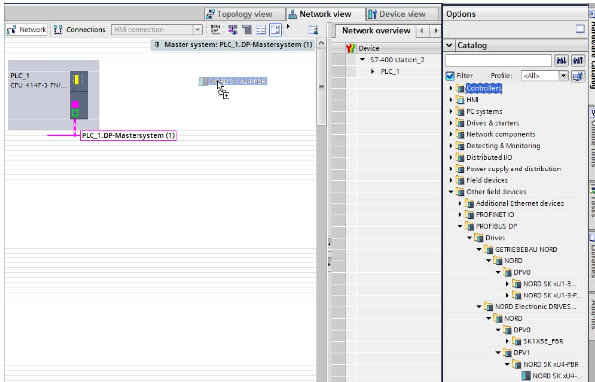
3. In the TIA device view, configure the slots for the specific application. For this, drag (insert) the modules from the hardware catalogue into the free slots of the bus interface. Existing modules can be deleted from the slots beforehand.
