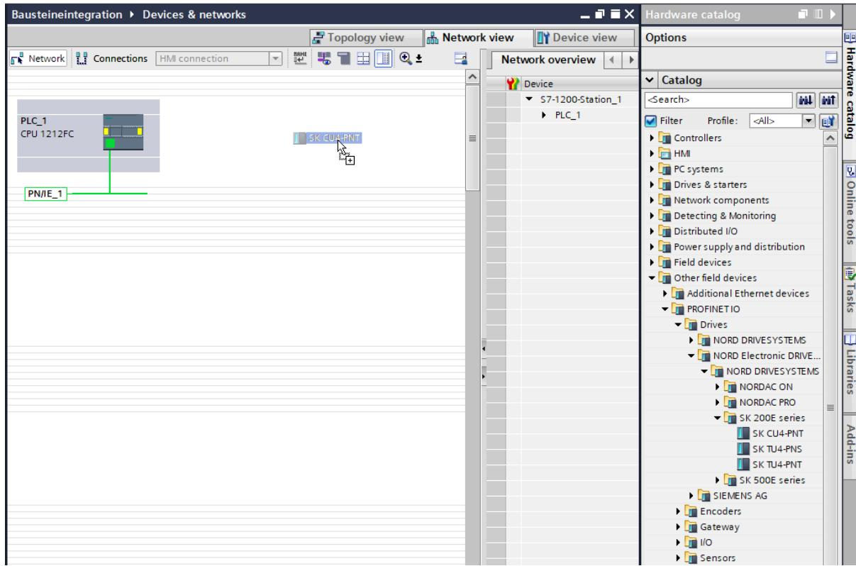
3. In the TIA device view, configure the slots for the specific application. For this, drag (insert) the modules from the hardware catalogue into the free slots of the bus interface. Existing modules can be deleted from the slots beforehand.
