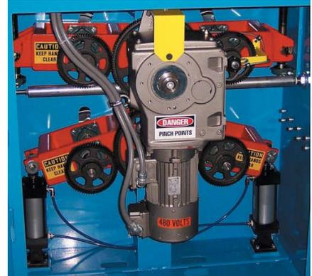
*Pipe puller showing NORD hollow shaft internal gearmotor with blower to achieve 1000:1 speed ratio.*
