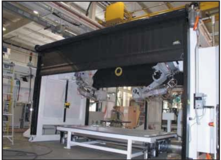
Once the UNIBLOC® gearmotor rolls the Guardian™ safety barrier into its closed and locked position, the robot starts its programmed cycle.
