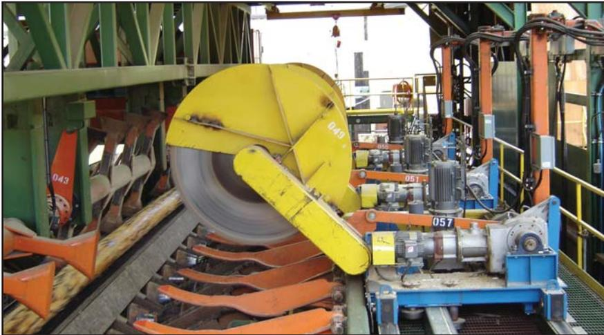
NORD Gear boxes control each of the 72-inch diameter saws.
