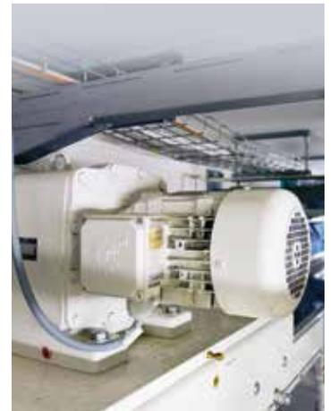
**Versatile.** – NORD geared motors drive agitators, mixers, grinders, pumps, and conveying systems.
