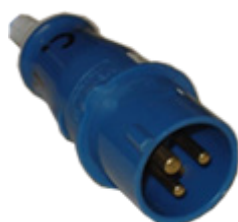
CEE AC plug connector 16 A, 230 V, L+N+PE, 6h, IP44
