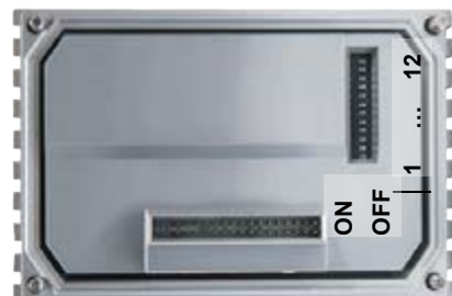
Factory settings DIP switches: OFF
