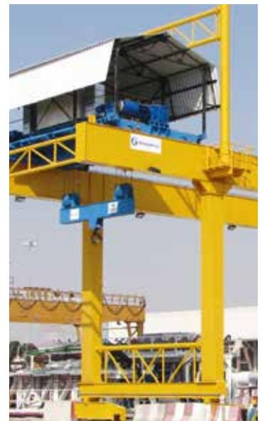
**Perfect balance.** – Synchronized hoist drives keep platforms riding in the shaft in a level position.
