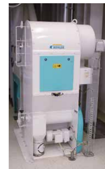
Grain cleaner. NORD driven screw conveyor removes low-density fraction in air-recycling aspirator.
