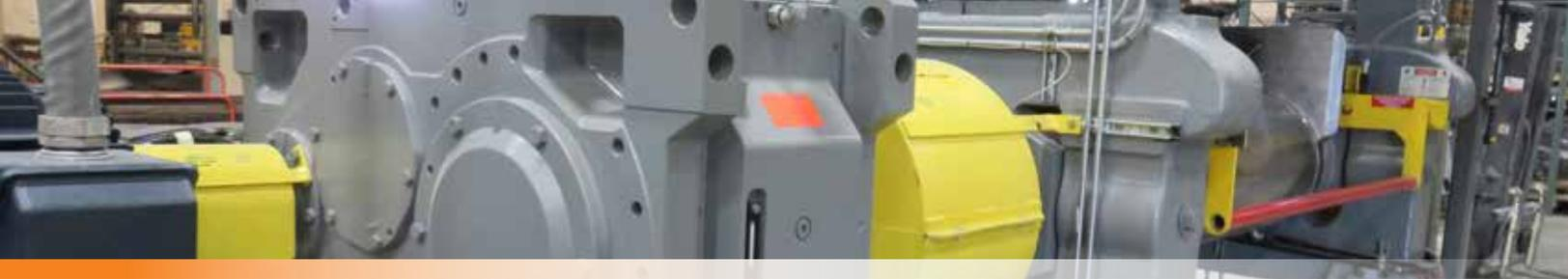
*Thermal load management required a central remote oil reservoir connected to the calander drive.* →
