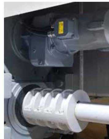
**Travelling drive.** – The BLOCK parallel shaft gear unit with helical gear first stage moves the turning machine over the saladin vat.
