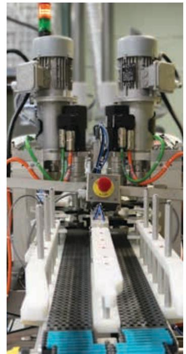
WGC mobile canning lines range from 2 to 4 fill heads and have a 27-42 can per minute filling capacity
