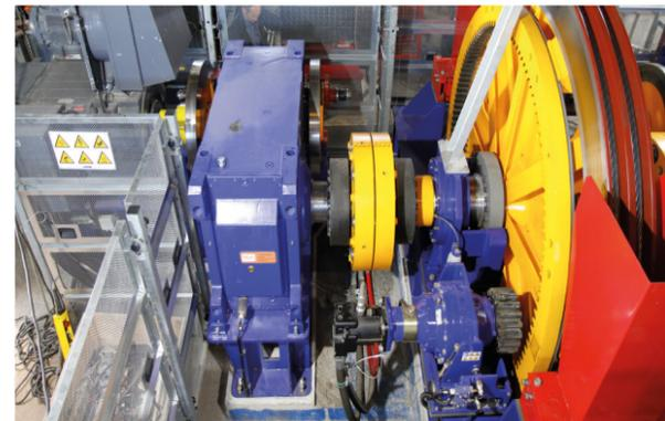
Two-stage industrial MAXXDRIVE™ parallel gear units
