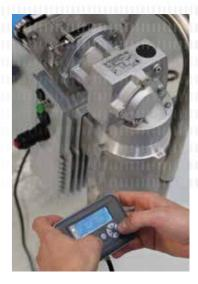
The motors are connected in series via via Profinet. This reduces the amount of cables and simplifies communication.
