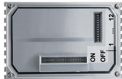
Factory settings DIP switches: OFF
