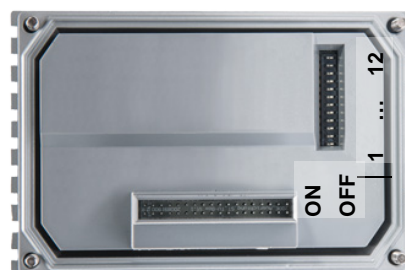
Factory settings DIP switches: OFF
