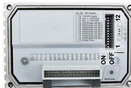
Factory settings DIP switches: OFF
