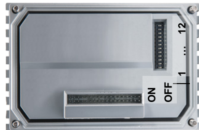
Factory settings DIP switches: OFF
