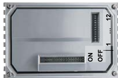
Factory settings DIP switches: OFF
