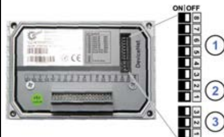
Factory settings DIP switches: OFF
