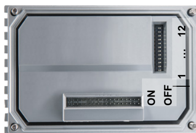
Factory settings DIP switches: OFF
