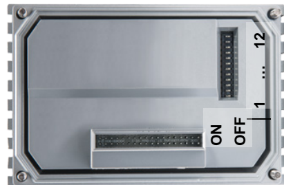
Factory settings DIP switches: OFF
