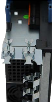
Detailed view of mounted EMC kits
