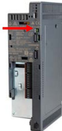
Remove the STO contact jumper.
