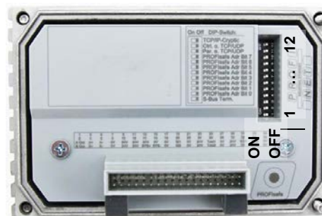
Factory settings DIP switches: OFF
